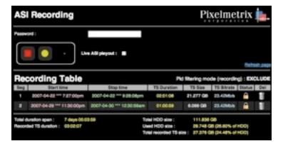
**Scheduled Recording:** Incoming transport streams can be recorded according to a pre-defined schedule, thereby making automation simpler.
